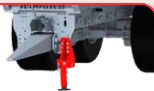
Hydraulic folding parking stand attached directly to the trailer chassis to free the drawbar and facilitate turning.
